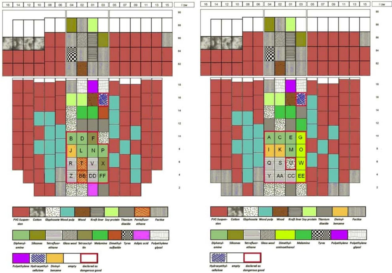
(Id. at 22, ¶ 31.) This diagram shows that in Hold 4, Tank J was surrounded on two sides by Tanks B and L, and diagonal to Tank D, all of which contained DPA. Similarly, Tank A—of heated DPA—was stored directly on top of the least insulated portion of Tank I, and Tank C was diagonal to it; Tank K had top, side, and diagonal DPA containers.
